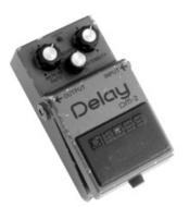
Analog echo units like the DM-2 were designed as improvements over the tape echoes that came before them, using "bucket brigade" electronics to give guitarists echo units that were more reliable than the tape-based delays, with the added advantage of a low-power circuit that can be run on batteries. Analog delays are treasured for the warm, distorted tones they produce, and this model based on the Boss<sup>®</sup> DM-2 gets you the same sort of thing in a new digital realm of existence.
