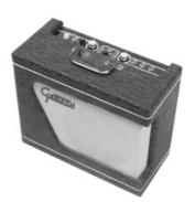
Another amp made by Valco/Supro<sup>®</sup>, this is the Gretsch<sup>®</sup> 6156. One of its curiosities is that the output transformer is actually mounted on its single 10-inch speaker, rather than on the amp chassis. It also has a lovely wraparound grill cloth, for a real futuristic look (or what passed for it in the '50s).
