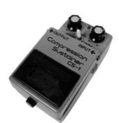
Roland®/Boss® jumped on the compressor stompbox bandwagon with the CS-1 Compression Sustainer. It has a fixed ratio, so this model based on it has the sustain control varying the threshold of the compressor circuitry. level does what you'd expect.
